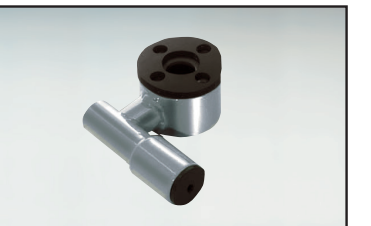
Release valve. Facilitates load releasing when large suction feet are used, for instance during vertical lifts. Available for standard as well as extended control unit.
